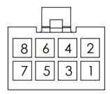
Terminal insertion end shown for ISMC housing (PDQ P/N 88850)
