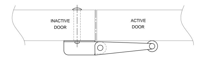
THE CARRY BAR WILL PUSH THE ACTIVE DOOR OPEN ALONG WITH THE INACTIVE DOOR AND ALLOW THE COORDINATOR MECHANISM TO ENGAGE BOTH DOORS AND TO COORDINATE THEM TO CLOSE CORRECTLY.
