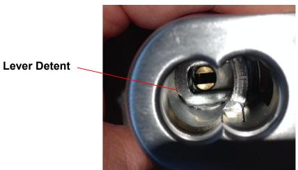
2. Insert a small flat tip screw driver into the IC opening in the lever
