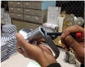
3. Insert the tip of the screw driver between the spring-loaded detent and the inner wall of the
