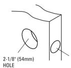
Drill 2-1/8" (54mm) hole through door face as marked for lockset. It is recommended that holes be drilled from both sides to prevent splitting. Drill 1" (25.4 mm) hole in center of door edge for latch.
