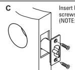
Insert latch and tighten screws.
